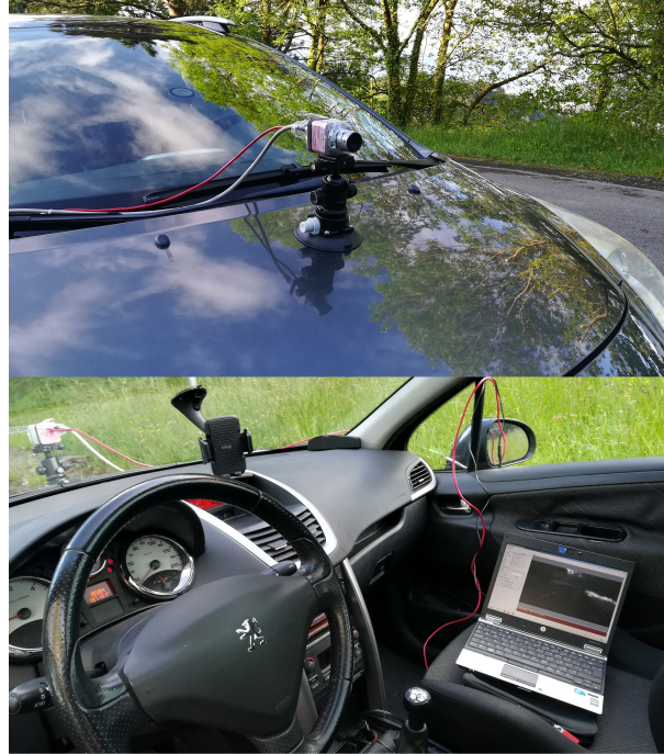
Figure 3.1: The Photonfocus snapshot HSI NIR camera mounted on a car
