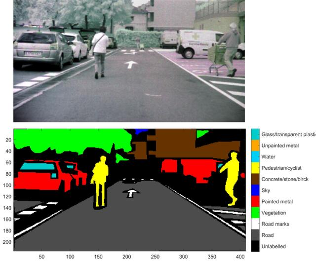
Fig. 2: False RGB image example (top) and ground-truth (bottom)
