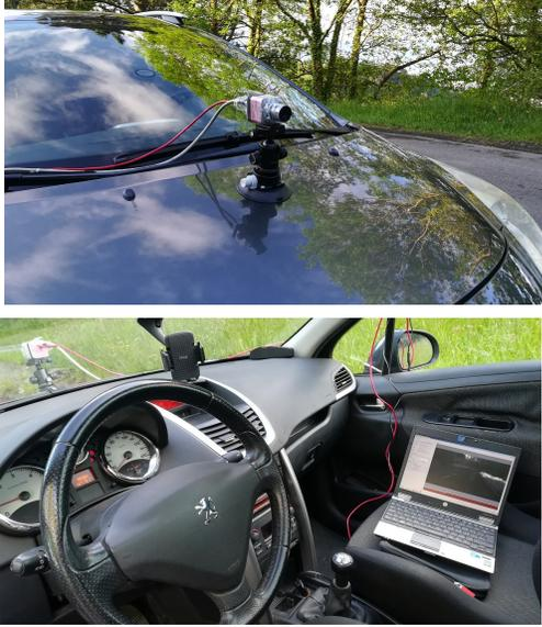
Fig. 1: The Photonfocus camera mounted on the front hood of the vehicle (top) and the recording laptop inside the car (bottom).
