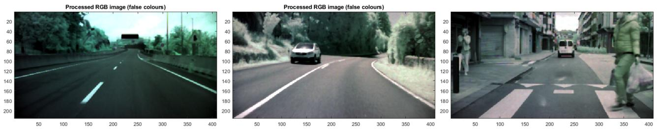
Fig. 3: False color example images generated from HSI cubes: a highway scene (left), a road scene (centre), and an urban scene (right)
